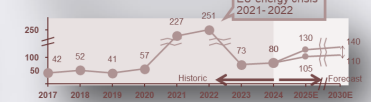
Electricity price is established based on the marginal costs of the most expensive powerplant meeting demand (gas fired powerplants).
